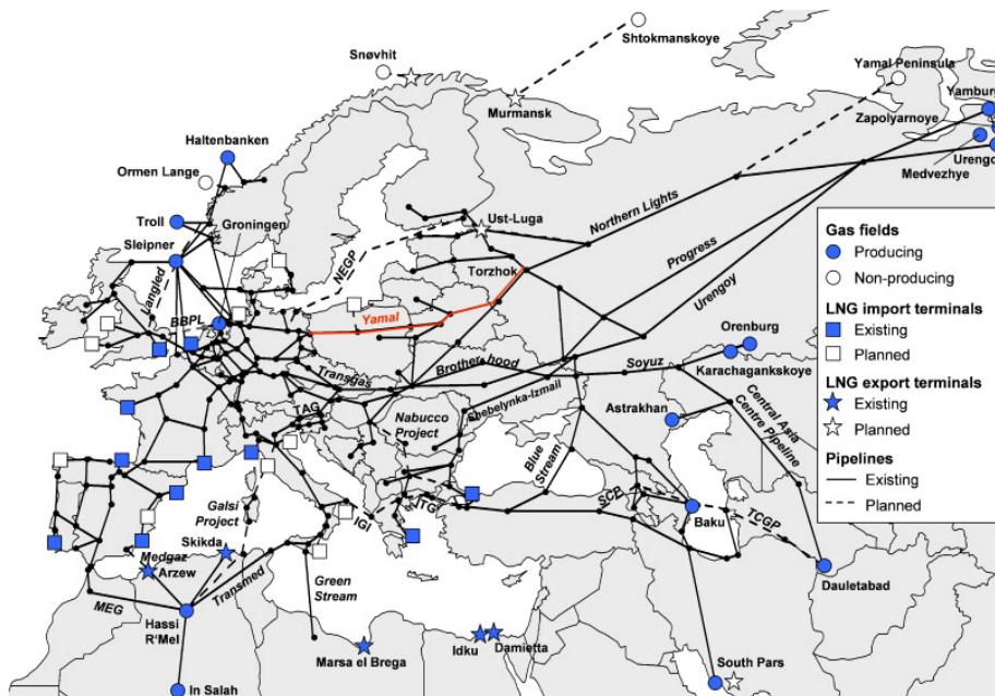
Figure 8. European gas network, and supply connections
